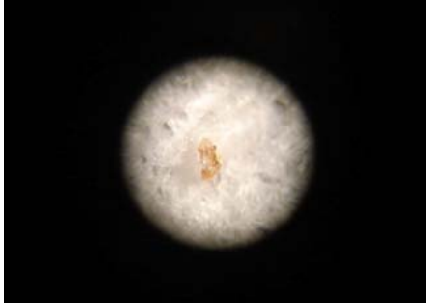
Visible Gold in drill core under microscope
